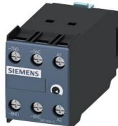
solid-state time-delayed front-side auxiliary switch Time range 0.5...10 s, 200 ... 240 V AC / DC, 1 NO contact, 1 NC contact OFF delay, without control signal for 3RT1
