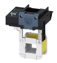
Withdrawable drive for contactors 3RT105, 3RT145 AC (50...60 Hz) / DC operation, 200 ... 277 V Operating mechanism: electronic with PLC input 24 V DC Screw terminal
