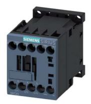
power contactor, AC-3e/AC-3, 7 A, 3 kW / 400 V, 1 NO, 100 V AC, 50 Hz 100-110 V, 60 Hz, 3-pole frame size S00, screw terminal
