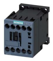
power contactor, AC-3e/AC-3, 7 A, 3 kW / 400 V, 3-pole, 208 V AC, 50/60 Hz, auxiliary contacts: 1 NO, screw terminal, size: S00,
