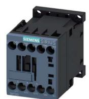
power contactor, AC-3e/AC-3, 7 A, 3 kW / 400 V, 1 NO, 110 V DC 3-pole, frame size S00 screw terminal
