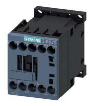
power contactor, AC-3e/AC-3, 7 A, 3 kW / 400 V, 3-pole, 24 V DC, 0.7-1.25\* Us, with integrated suppressor diode, auxiliary contacts: 1 NC, screw terminal, size: S00, suitable for PLC outputs, not expandable with auxiliary switch
