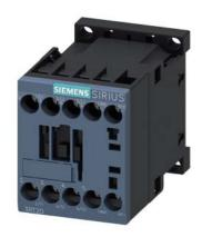
power contactor, AC-3e/AC-3, 7 A, 3 kW / 400 V, 3-pole, 24 V DC,  $0.85-1.85^{*}$  Us, auxiliary contacts: 1 NO, screw terminal, size: S00, not expandable with auxiliary switch
