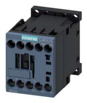
power contactor, AC-3e/AC-3, 7 A, 3 kW / 400 V, 3-pole, 24 V DC, 0.85-1.85 $^{\star}$  Us, auxiliary contacts: 1 NC, screw terminal, size: S00, not expandable with auxiliary switch
