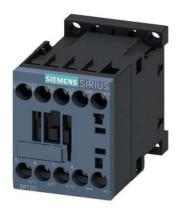
power contactor, AC-3e/AC-3, 7 A, 3 kW / 400 V, 1 NC, 24 V DC 0.85-1.85  $^{\star}$  US, with diode integrated, 3-pole, frame size S00, screw terminal not expandable with auxiliary switch
