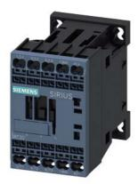
power contactor, AC-3e/AC-3, 7 A, 3 kW / 400 V, 1 NO, 110 V DC 3-pole, frame size S00 spring-loaded terminal
