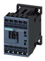
power contactor, AC-3e/AC-3, 7 A, 3 kW / 400 V, 3-pole, 24 V DC, 0.85-1.85\* Us, auxiliary contacts: 1 NO, spring-loaded terminal, size: S00, not expandable with auxiliary switch
