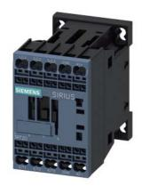
power contactor, AC-3e/AC-3, 7 A, 3 kW / 400 V, 3-pole, 24 V DC, 0.85-1.85\* Us, with integrated diode, auxiliary contacts: 1 NC, spring-loaded terminal, size: S00, not expandable with auxiliary switch
