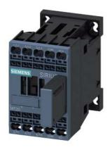
power contactor, AC-3e/AC-3, 7 A, 3 kW / 400 V, 3-pole, 24 V DC, 0.85-1.85\* Us, with varistor plugged on, auxiliary contacts: 1 NC, spring-loaded terminal, size: S00, not expandable with auxiliary switch
