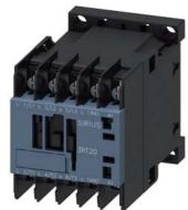
power contactor, AC-3e/AC-3, 7 A, 3 kW / 400 V, 3-pole, 100 V AC, 50 Hz / 100-110 V, 60 Hz, auxiliary contacts: 1 NO, ring cable lug connection, size: S00  $\,$
