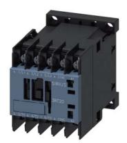
power contactor, AC-3e/AC-3, 7 A, 3 kW / 400 V, 3-pole, 100 V AC, 50 Hz / 100-110 V, 60 Hz, auxiliary contacts: 1 NC, ring cable lug connection, size: S00
