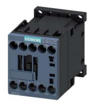
power contactor, AC-3e/AC-3, 9 A, 4 kW / 400 V, 3-pole, 120 V AC, 50/60 Hz, auxiliary contacts: 1 NO, screw terminal, size: S00  $\,$
