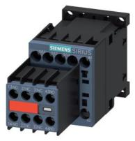
power contactor, AC-3e/AC-3, 9 A, 4 kW / 400 V, 2 NO+2 NC 110 V AC, 50 Hz 120 V, 60 Hz 3-pole, frame size S00 screw terminal captive auxiliary switch
