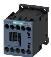
power contactor, AC-3e/AC-3, 9 A, 4 kW / 400 V, 1 NC, 200 V AC, 50 Hz 200-220 V, 60 Hz, 3-pole, frame size S00, screw terminal
