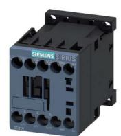
power contactor, AC-3e/AC-3, 9 A, 4 kW / 400 V, 3-pole, 24 V DC, auxiliary contacts: 1 NO, screw terminal, size: S00, upright mounting position
