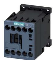
power contactor, AC-3e/AC-3, 9 A, 4 kW / 400 V, 1 NO, 72 V DC 3-pole, frame size S00 screw terminal
