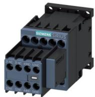
power contactor, AC-3e/AC-3, 9 A, 4 kW / 400 V, 3-pole, 120 V AC, 50/60 Hz, with varistor plugged on, auxiliary contacts: 3 NO + 2 NC, screw terminal, size: S00, removable auxiliary switch
