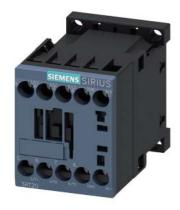
power contactor, AC-3e/AC-3, 9 A, 4 kW / 400 V, 3-pole, 24 V DC, 0.7-1.25\* Us, with integrated suppressor diode, auxiliary contacts: 1 NC, screw terminal, size: S00, suitable for PLC outputs, not expandable with auxiliary switch
