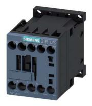
power contactor, AC-3e/AC-3, 9 A, 4 kW / 400 V, 3-pole, 24 V DC,  $0.85-1.85^{*}$  Us, auxiliary contacts: 1 NC, screw terminal, size: S00, not expandable with auxiliary switch
