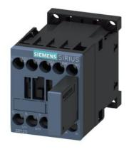
power contactor, AC-3e/AC-3, 9 A, 4 kW / 400 V, 3-pole, 24 V DC, 0.7-1.25\* Us, with varistor plugged on, auxiliary contacts: 1 NC, screw terminal, size: S00, not expandable with auxiliary switch
