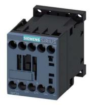
power contactor, AC-3e/AC-3, 9 A, 4 kW / 400 V, 1 NC, 24 V DC 0.85-1.85  $^{\star}$  US, with diode integrated, 3-pole, frame size S00, screw terminal not expandable with auxiliary switch
