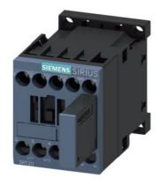
power contactor, AC-3e/AC-3, 9 A, 4 kW / 400 V, 3-pole, 24 V DC, 0.85-1.85\* Us, with varistor plugged on, auxiliary contacts: 1 NO, screw terminal, size: S00, not expandable with auxiliary switch
