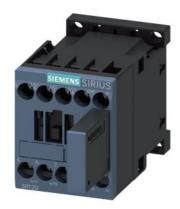
power contactor, AC-3e/AC-3, 9 A, 4 kW / 400 V, 3-pole, 24 V DC, 0.85-1.85\* Us, with varistor plugged on, auxiliary contacts: 1 NC, screw terminal, size: S00, not expandable with auxiliary switch
