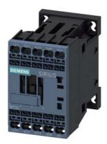
power contactor, AC-3e/AC-3, 9 A, 4 kW / 400 V, 1 NC, 125 V DC, 3-pole, frame size S00 spring-loaded terminal
