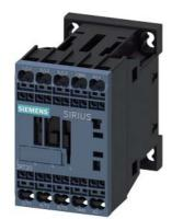
power contactor, AC-3e/AC-3, 9 A, 4 kW / 400 V, 3-pole, 24 V DC, 0.7-1.25\* Us, with integrated suppressor diode, auxiliary contacts: 1 NO, spring-loaded terminal, size: S00, suitable for PLC outputs, not expandable with auxiliary switch
