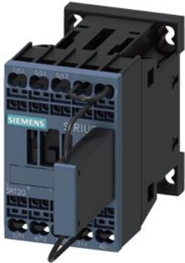
traction contactor, AC-3e/AC-3, 9 A, 4 kW / 400 V, 72 V DC 0.7-1.25\* US, with varistor integrated, 3-pole, frame size S00, spring-loaded terminal
