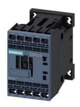
power contactor, AC-3e/AC-3, 9 A, 4 kW / 400 V, 3-pole, 24 V DC,  $0.85-1.85^*$  Us, auxiliary contacts: 1 NC, spring-loaded terminal, size: S00, not expandable with auxiliary switch
