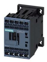
power contactor, AC-3e/AC-3, 9 A, 4 kW / 400 V, 3-pole, 24 V DC, 0.85-1.85\* Us, with integrated suppressor diode, auxiliary contacts: 1 NO, spring-loaded terminal, size: \$00
