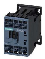
power contactor, AC-3e/AC-3, 9 A, 4 kW / 400 V, 1 NC, 24 V DC varistor integrated, 3-pole, spring-loaded terminal
