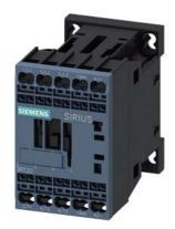
power contactor, AC-3e/AC-3, 9 A, 4 kW / 400 V, 3-pole, 24 V DC, 0.85-1.85\* Us, with integrated diode, auxiliary contacts: 1 NO, spring-loaded terminal, size: S00, not expandable with auxiliary switch
