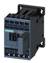
power contactor, AC-3e/AC-3, 9 A, 4 kW / 400 V, 3-pole, 24 V DC,  $0.85\text{-}1.85^{*}$  Us, with varistor plugged on, auxiliary contacts: 1 NC, spring-loaded terminal, size: S00, not expandable with auxiliary switch
