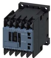
power contactor, AC-3e/AC-3, 9 A, 4 kW / 400 V, 3-pole, 100 V AC, 50 Hz / 100-110 V, 60 Hz, auxiliary contacts: 1 NO, ring cable lug connection, size: S00  $\,$
