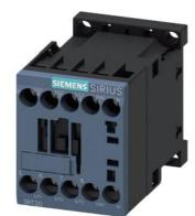
power contactor, AC-3e/AC-3, 12 A, 5.5 kW / 400 V, 3-pole, 100 V AC, 50 Hz / 100-110 V, 60 Hz, auxiliary contacts: 1 NC, screw terminal, size: S00
