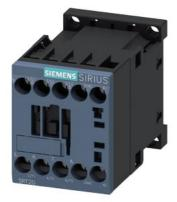
power contactor, AC-3e/AC-3, 12 A, 5.5 kW / 400 V, 1 NC, 110 V AC, 50 Hz, 120 V 60 Hz, 3-pole, frame size S00 screw terminal
