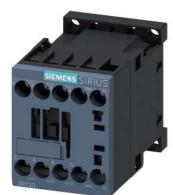
power contactor, AC-3e/AC-3, 12 A, 5.5 kW / 400 V, 1 NO, 200 V AC, 50 Hz 200-220 V, 60 Hz, 3-pole frame size S00, screw terminal
