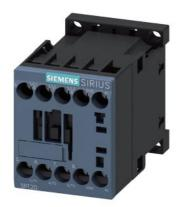
power contactor, AC-3e/AC-3, 12 A, 5.5 kW / 400 V, 1 NC, 200 V AC, 50 Hz 200-220 V, 60 Hz, 3-pole frame size S00, screw terminal
