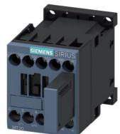
power contactor, AC-3e/AC-3, 12 A, 5.5 kW / 400 V, 1 NO, 24 V DC 0.7-1.25\* Us, with varistor plugged on, 3-pole frame size S00, screw terminal not expandable with auxiliary switch
