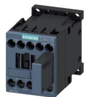
power contactor, AC-3e/AC-3, 12 A, 5.5 kW / 400 V, 1 NC, 24 V DC 0.7-1.25\* Us, with varistor plugged on, 3-pole frame size S00, screw terminal not expandable with auxiliary switch
