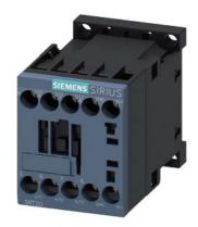
power contactor, AC-3e/AC-3, 12 A, 5.5 kW / 400 V, 3-pole, 24 V DC, 0.85-1.85  $^{\star}$  Us, with integrated diode, auxiliary contacts: 1 NC, screw terminal, size: S00, not expandable with auxiliary switch
