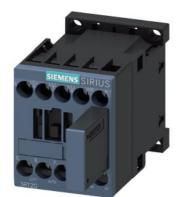
power contactor, AC-3e/AC-3, 12 A, 5.5 kW / 400 V, 3-pole, 24 V DC, 0.85-1.85\* Us, with varistor plugged on, auxiliary contacts: 1 NC, screw terminal, size: S00, not expandable with auxiliary switch
