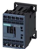
power contactor, AC-3e/AC-3, 12 A, 5.5 kW / 400 V, 1 NO, 110 V AC, 50 Hz, 120 V 60 Hz, 3-pole, frame size S00 spring-loaded terminal
