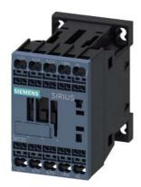
power contactor, AC-3e/AC-3, 12 A, 5.5 kW / 400 V, 1 NO, 220 V AC, 50 / 60 Hz 3-pole, frame size S00 spring-loaded terminal
