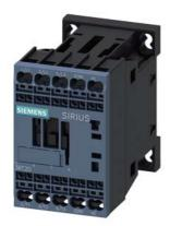
power contactor, AC-3e/AC-3, 12 A, 5.5 kW / 400 V, 1 NC, 220 V AC, 50 Hz 240 V, 60 Hz, 3-pole frame size S00, spring-loaded terminal
