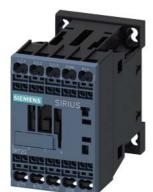
power contactor, AC-3e/AC-3, 12 A, 5.5 kW / 400 V, 1 NC, 24 V DC 3-pole, frame size S00 spring-loaded terminal upright mounting position
