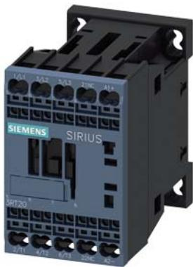
power contactor, AC-3e/AC-3, 12 A, 5.5 kW / 400 V, 3-pole, 12 V DC, 0.7-1.25\* Us, with integrated suppressor diode, auxiliary contacts: 1 NC, spring-loaded terminal, size: S00, suitable for PLC outputs, not expandable with auxiliary switch
