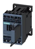
traction contactor, AC-3e/AC-3, 12 A, 5.5 kW / 400 V, 24 V DC, 0.7-1.25\*Us with integrated suppressor diode 3-pole, frame size S00 spring-loaded terminal suitable for PLC outputs for upright mounting position not expandable with auxiliary switch
